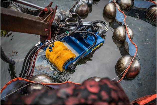
3 July 2017, Lamor bucket skimmer inside Desmi Pyroboom collecting burn residue
